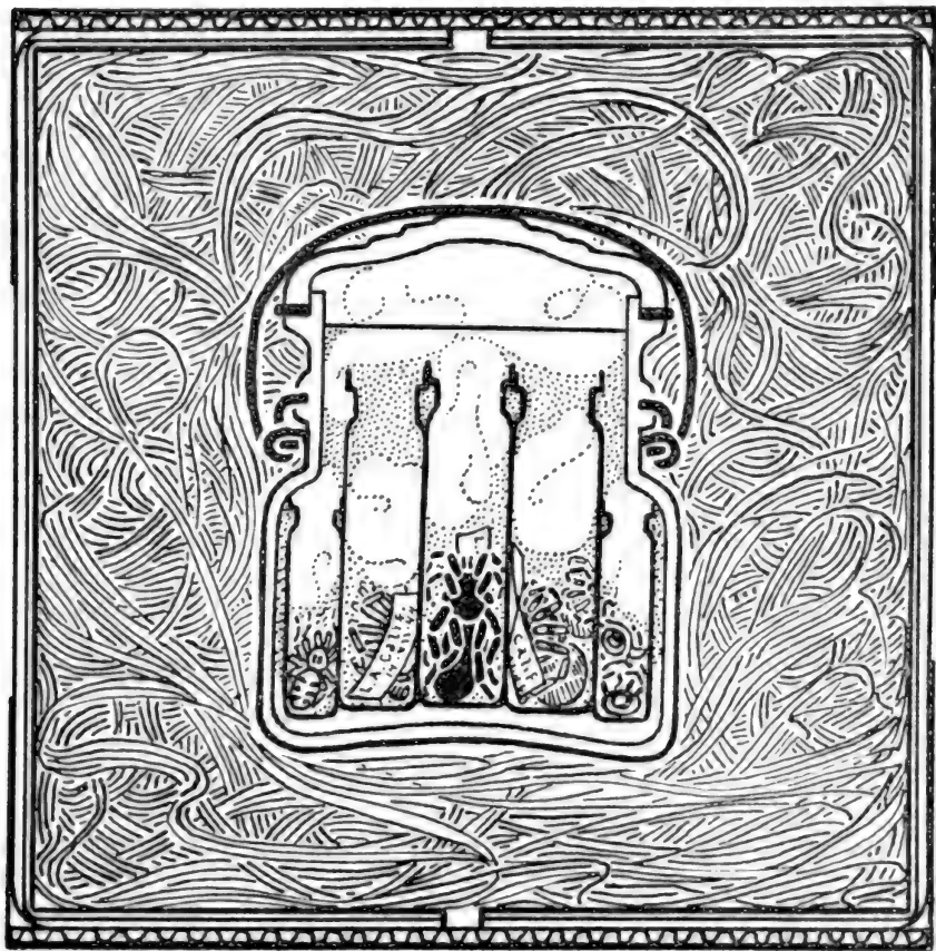
Fig. 15. Diagram of a jar of alcoholic specimens packed for shipping.
